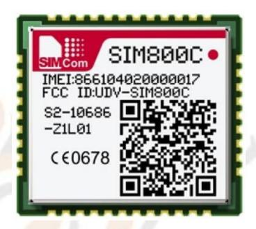
SIM 800C Module is a complete Quad-band GSM/GPRS solution in a SMT type, which can be embedded in the customer applications.
