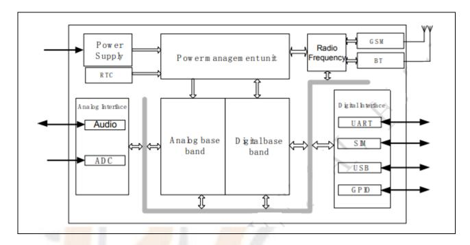
The following figure shows a functional diagram of SIM800C:
