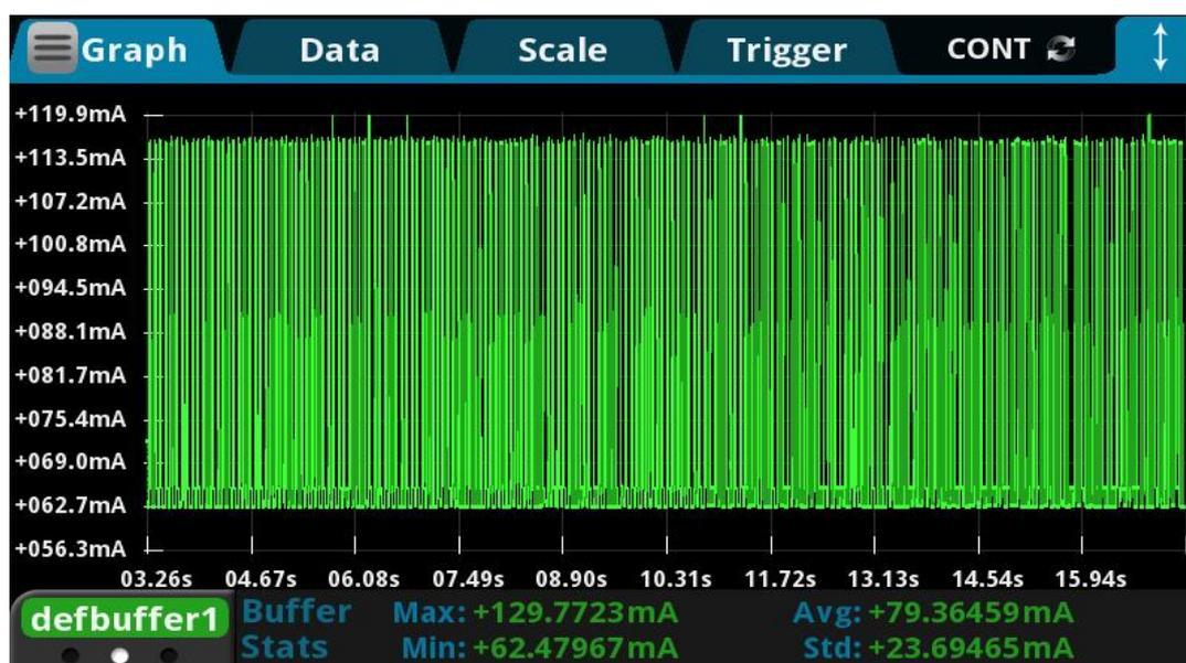
Figure 11 Measured data of module working current
