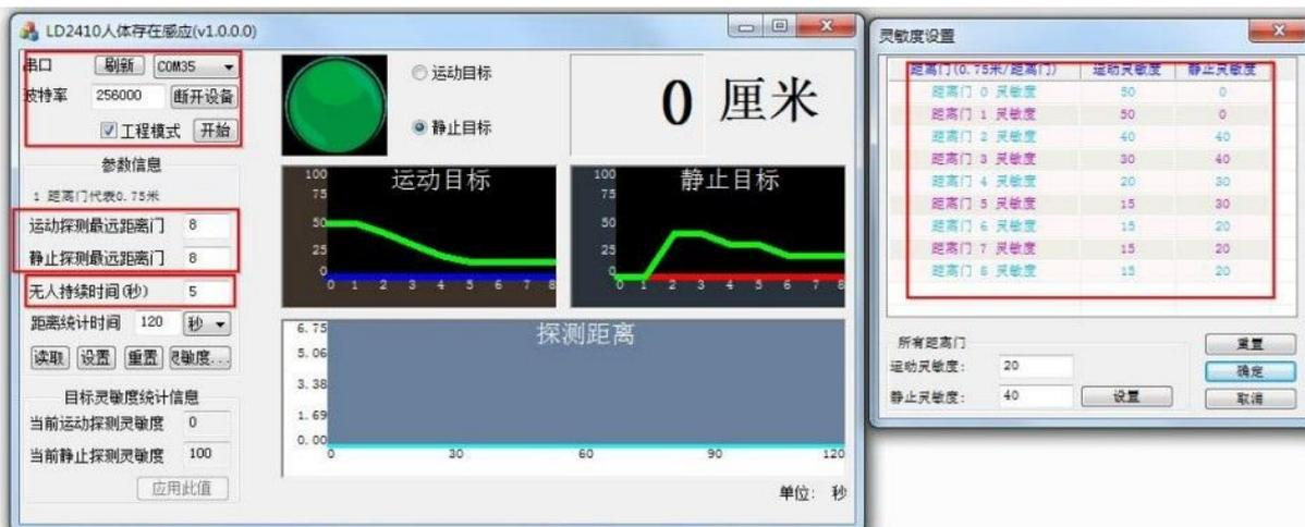
The ball is the target status output indication: **red** means there is a moving target; **purple** means there is a stationary target; **green** means no one.
