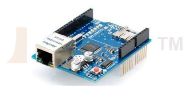
The Arduino Ethernet Shield allows an Arduino board to connect to the internet. It is based on the Wiznet W5100 ethernet chip. The Wiznet W5100 provides a network (IP) stack capable of both TCP and UDP. The Ethernet W5100 Shield Network Expansion Board w/ Micro SD Card Slot supports up to four simultaneous socket connections.
