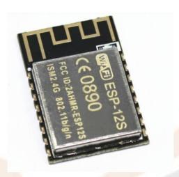
Ai Thinker ESP-12S ESP8266 Serial WiFi Module has a highly competitive package size and ultra-low power technology. ESP-12S can be widely used in a variety of networking, for home automation, industrial wireless control, baby monitors, wearable electronic products, wireless location sensing devices, and wireless positioning system signals.
