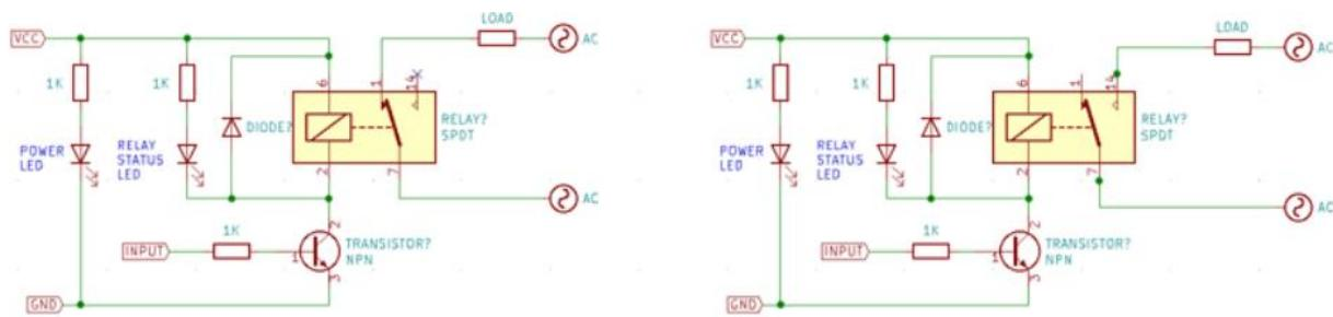
For simple on/off applications, the relay can be connected as shown above. One terminal of mains is connected to common, and the other is connected to NO or NC depending on whether the load should be connected/ disconnected when the relay is active.
