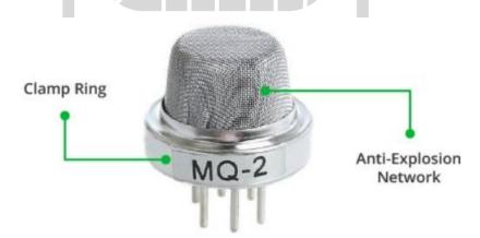
It also protects the sensor and filters out suspended particles, allowing only gaseous elements to pass through the chamber. A copper-plated clamping ring secures the mesh to the rest of the body.
