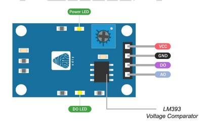
The module includes a potentiometer for adjusting the sensitivity of the digital output (D0). You can use it to set a threshold so that when the gas concentration exceeds the threshold value, the module outputs LOW otherwise HIGH.
