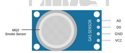
VCC: Supplies power to the module. Connect it to the 5V output of your Arduino.
